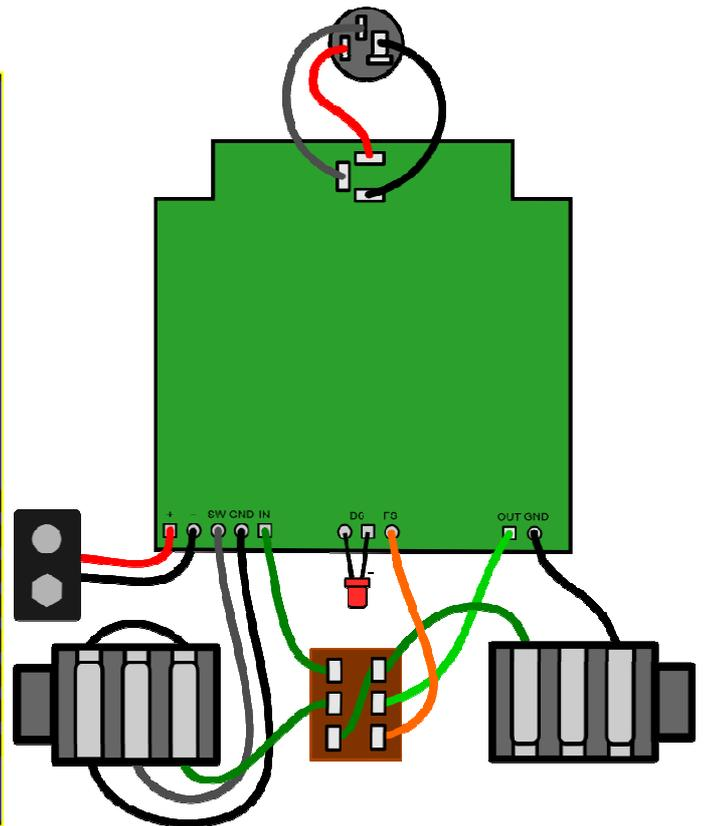
Fig. 3: Wiring diagram (with millennium bypass)
