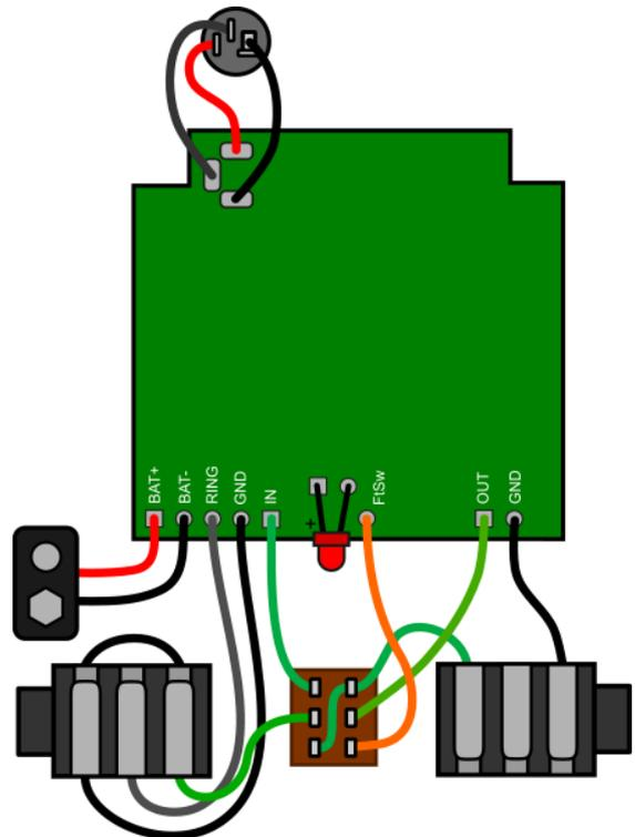
Fig. 3: Wiring diagram (with millennium bypass)
