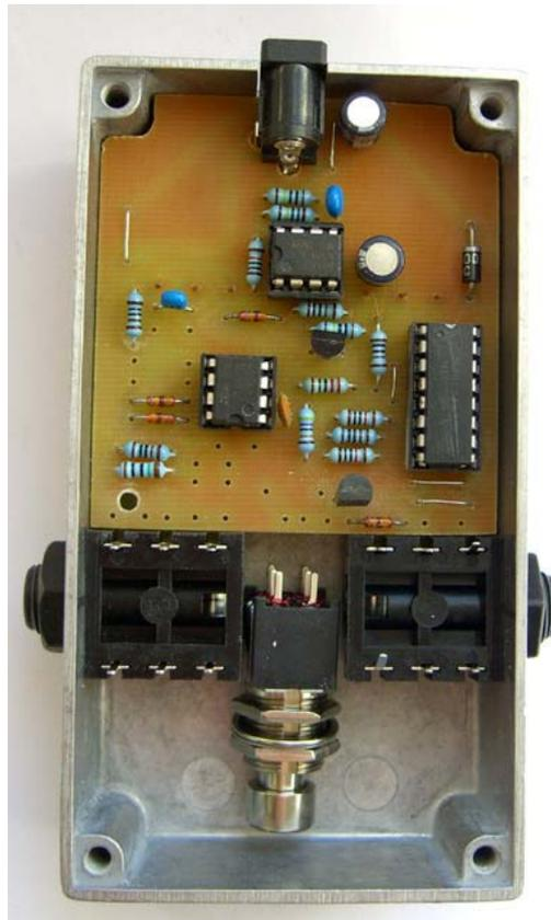
Now I drill the hole for the footswitch. I drill the hole slightly smaller than it needs to be and then file out the rest, leaving a tab or key that fits into the notch on the switch. This might seem like a pain, but it means you can tighten the fixing nut without having to hold the body of the switch at the same time since the key/notch stops the switch from rotating. If you don't do this then there is a good chance you'll break the switch while it is twisting (I've done it).
