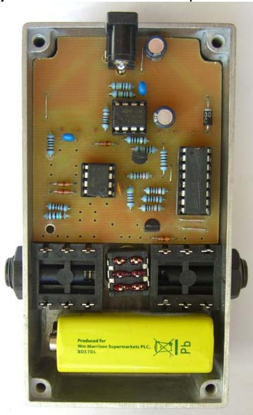
Now I do the off board wiring, keeping everything as short as possible. Bare in mind that when installing the whole assembly into the enclosure the footswitch must go in *after* the jacks, so its wiring needs to have some slack. I pass the battery wires through a hole in the PCB which provides some strain relief for the solder joints, as shown in the right-hand photo.
