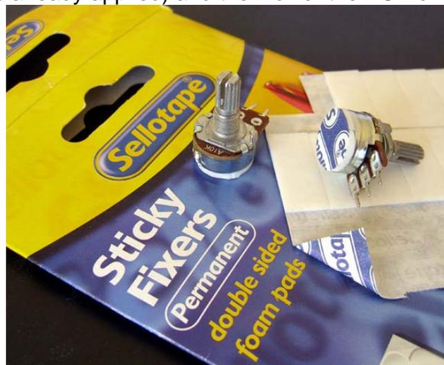
Then I wire the pots to the PCB. Also, if I need to ground the enclosure I usually do it by soldering a wire from the ground plane to one of the pots, as shown in the right-hand photo (it helps to put some solder onto the body of the pot *before* sticking the pot to the PCB!).
