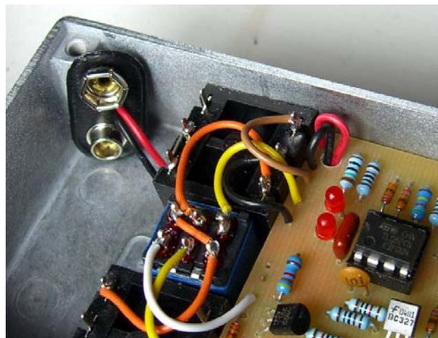
I usually drill the hole for the LED last of all, positioning it by eye; bending the legs a bit to make it slot into place is not a problem. Once the LED is seated, I solder it in place.
